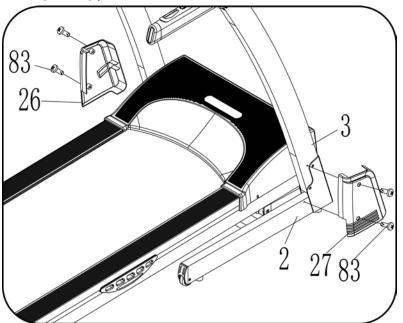
Use wrench screw(12) diver, lock the base covers(26/27) onto the base frame with bolt ST4.2\*19(83).
