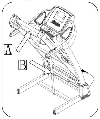
Pull up the base frame at position A, till hearing the sound that the air pressure bar B is locked into the round tube
