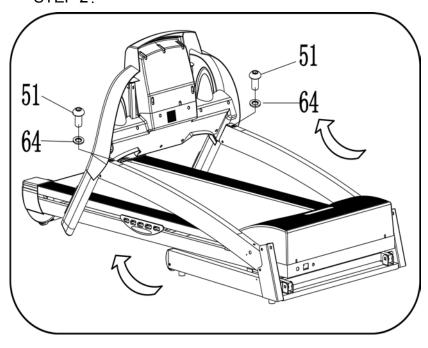
Folding the computer, use 5# Allen wrench, lock the computer onto the L&R upright tubes with the boltM8\*16(51) and lock washer(64). Notice:On both sides of the height is the same.
